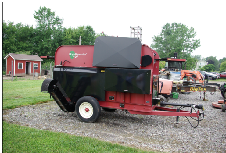
A Hops Harvester used to separate the hops from the vine
